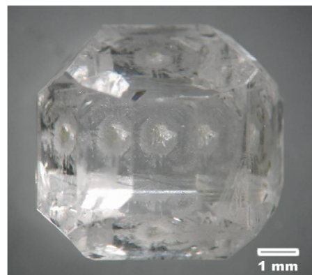
Figure 5. A type IIa diamond grown at optimal conditions; multiple reflections of the seed interface are visible through the top face of the crystal.
